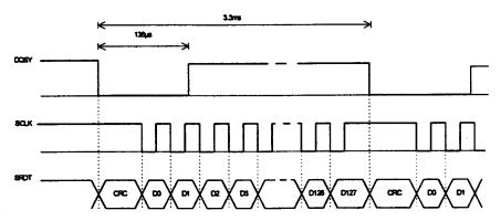
Signal DQSY is used as an interrupt input signal for the microcontroller. After the falling edge of DQSY the microcontroller sends the clock signal 'SCLK'. The serial data is then read synchronously to this clock signal into the microcontroller.
