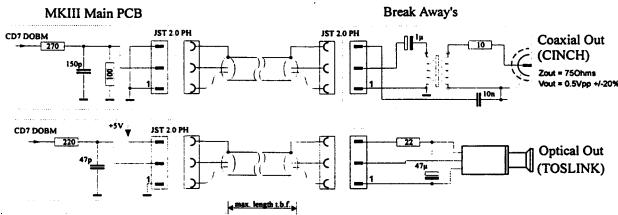
Digital out can be realized as either coaxial- or optical-output. For reaching the required accuracy of the clock signal, the ceramic resonator is replaced by a crystal.
