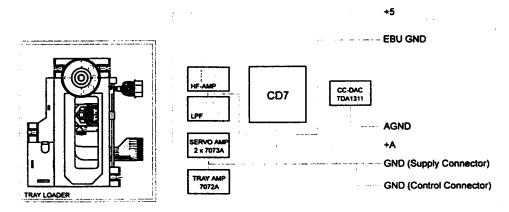
The next figure shows supply and grounding concept of ECO-SL MKIII with IIS-Interface
